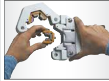
The die snaps quickly into the press fixture requiring no pins or screws.
