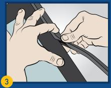
Apply with one hand, securing with the other; apply molding at 45° angle at point of contact
