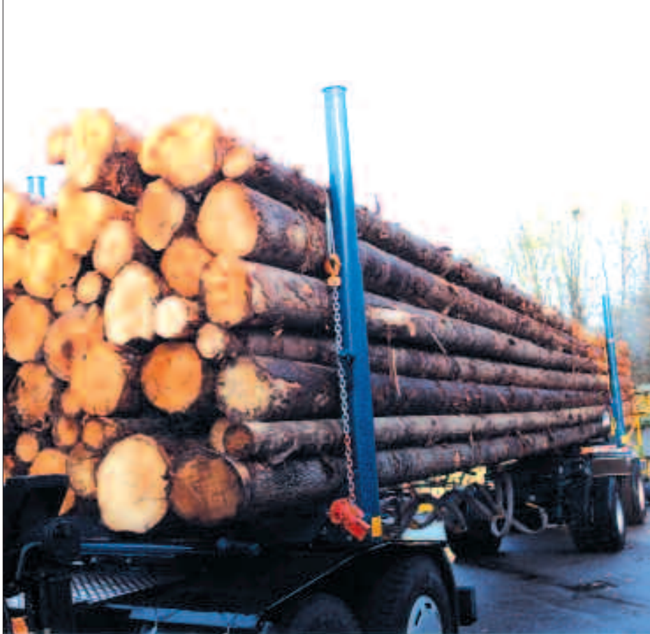
Lashing wire rope and ratchet lever hoist as tensioner elements
