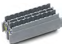
FH360 Mini blade fuse box. Accepts 20 mini blade fuses. This fuse box can be mounted using any of the modular frames above. Supplied complete with terminal locking bars and 40 terminals for crimping cables 1.0mm 2 to 2.0mm 2 . Individually packed.
